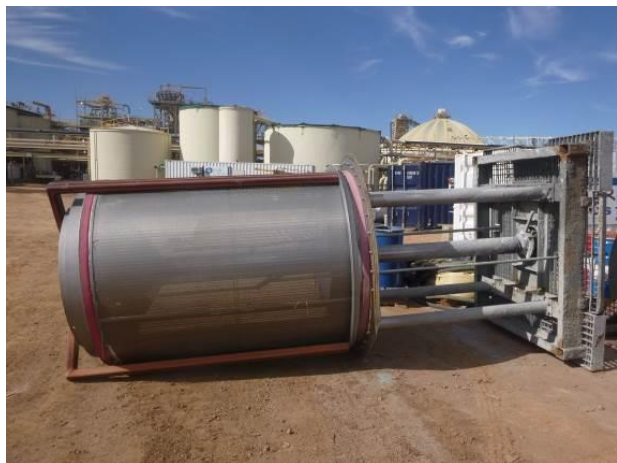
Figure 11 –Stainless steel carbon transfer screen
