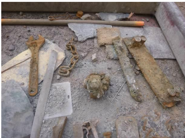
Figure 3 – Various items that have been removed from inside of a tank once drained. Larger items such as an interstage screen and agitator blades have been known
