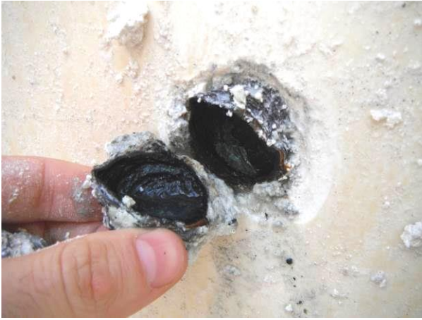
Figure 9 – Stereotypical MIC tubercle formation on the inside of a tank
