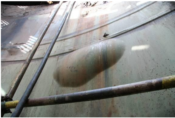
Figure 1 - Example of an osmotic blister and subsequent underfilm adhesion failure
