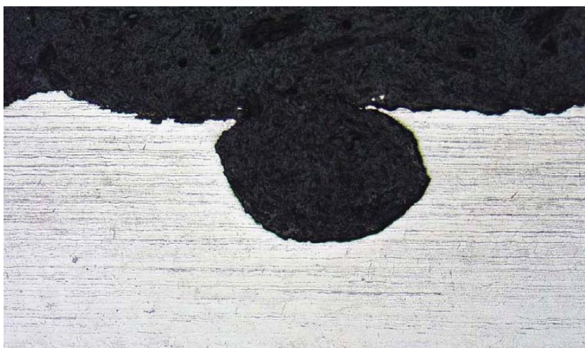
Fig. 2C – General view of the pit morphology under magnification (x100) at the pipe bore, with the narrow opening and smooth, rounded internal surface..
