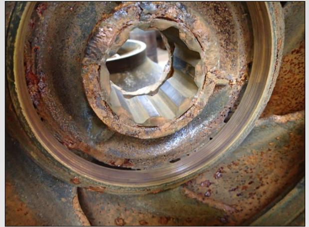
Failures occur due to numerous reasons: It can be the result of design, where materials and shapes are not appropriate for the application. Failure can also be partly the result of operation and process, where the required procedures were not properly applied throughout the whole process. In most cases, failures that are the result of corrosion occur due to the **chemical, electro-chemical and microbial degradation mechanisms.**
